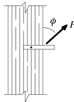
b) Connector installed perpendicular to grain
