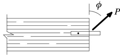
a) Connector installed parallel to grain
