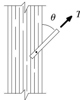
Figure 1 — Angle to grain installation of connector with tension loading
